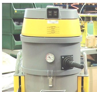
Mechanical filter shaker and vacuum gauge
